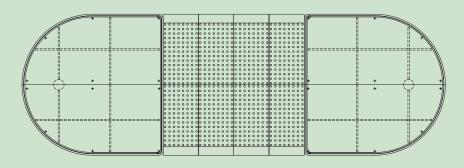
All of the Rosehill Traffic Islands can be configured to form a pedestrian refuge island, incorporating surface mounted, 'blister' pattern tactile paving.
