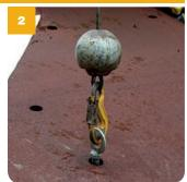
» Screw the lifting eye supplied into the centre hole until fully tight. Locate straps or chain through the eye ready for lifting.
